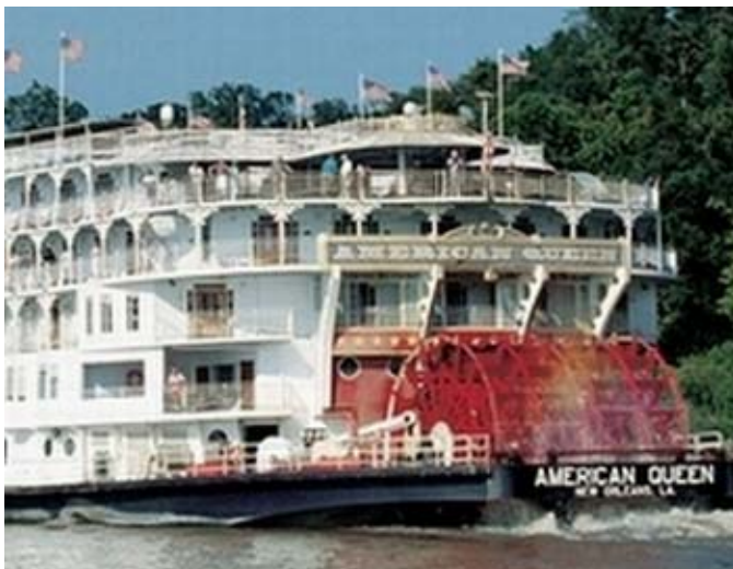
The American Queen’s 45 ton Paddle-Wheel, Run by a Steam-Diesel-Electric “Z” drive
